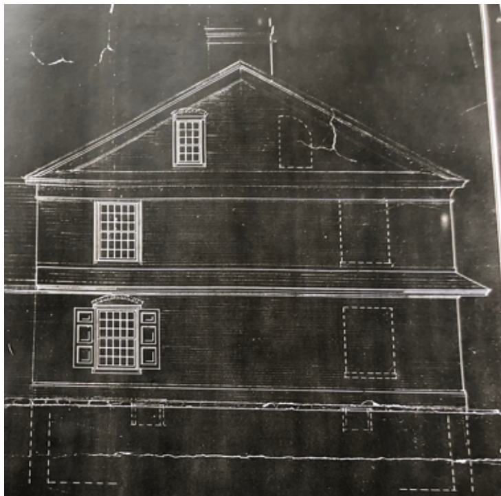
West Gable Elevation. The dashed figures indicate infills. The pent eve and cove molding were restored fitting to the scars on the brick face.
