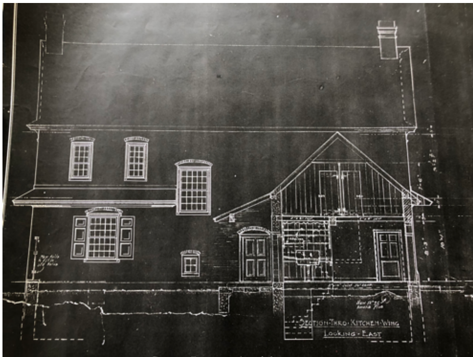
North Gable Elevation. Included is a proposed attached kitchen. This kitchen design was not implemented.
